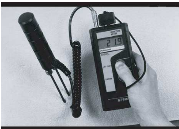
Fig. 4. Professional Pin Meter With Deep Wall Probe.
